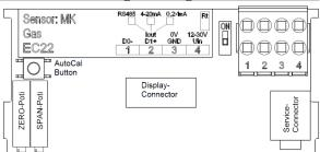
If the button is already released during the 1st phase, i.e. too early, then no adjustment is made and the measuring operation is continued as normal.
