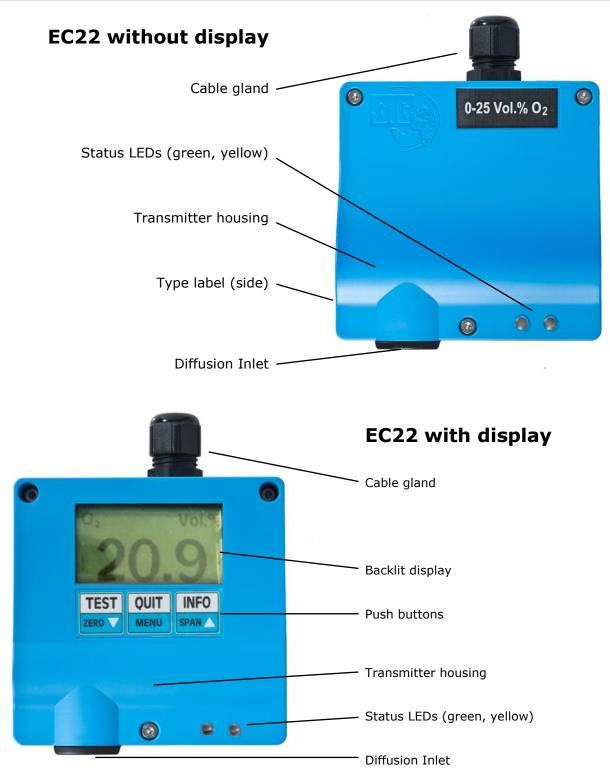
The transmitter housing contains the gas sensor and the transmitter electronics. The electronics converts the measuring signal into a gas concentration which is then signaled via an analog current signal of 4-20 mA or 0.2-1 mA or a digital RS-485 bus signal using the Modbus RTU protocol. In the display variant, gas concentration and status information are displayed.
