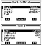
Alarm1 to Alarm3: Selection of the alarm limit value to be configured.
